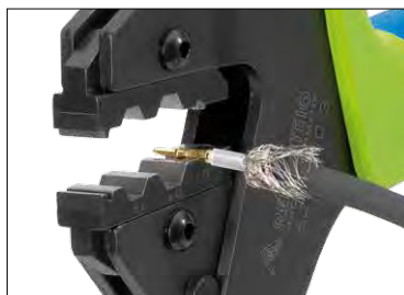
Innenleiter-Crimp Inner conductor crimp
